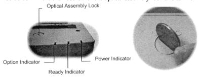
Before attempting to transport your scanner, it is important that you lock the optical assembly in place to avoid any possible damage to the scanner's optical components. To lock the optical assembly, insert a coin and turn it until points to the lock mark.
